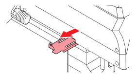
5 Hold the handle on the waste ink tank and slide out.
