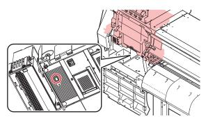
5 Once cleaning is complete, close the maintenance covers, then press the [ENTER] key.
