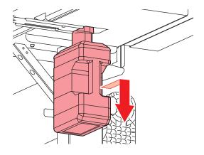
Attach the cap to the removed waste ink tank, and use tape to prevent leakage of waste ink.
