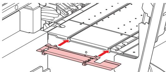
**7** Secure the media holder stopper with the screw.
