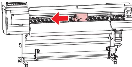
**3 Turn off the power.****4 Open the front cover.****5 Remove the cap absorber.**
