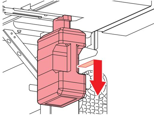
**6** Attach the cap to the removed waste ink tank, and use tape to prevent leakage of waste ink.
