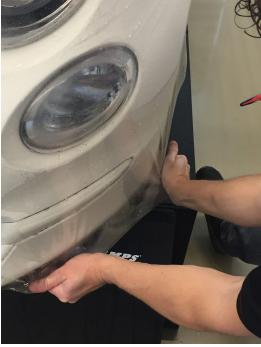
Conventional convex and compound shapes on car fronts are mostly suitable to be covered with all the paint protection films in the Avery Dennison SPF series, but in some deeper corrugated shapes it may be necessary to make an incision in order to avoid any form of air/water entrapment in the deep recesses. This incision does not jeopardize the functionality or durability of the product.
